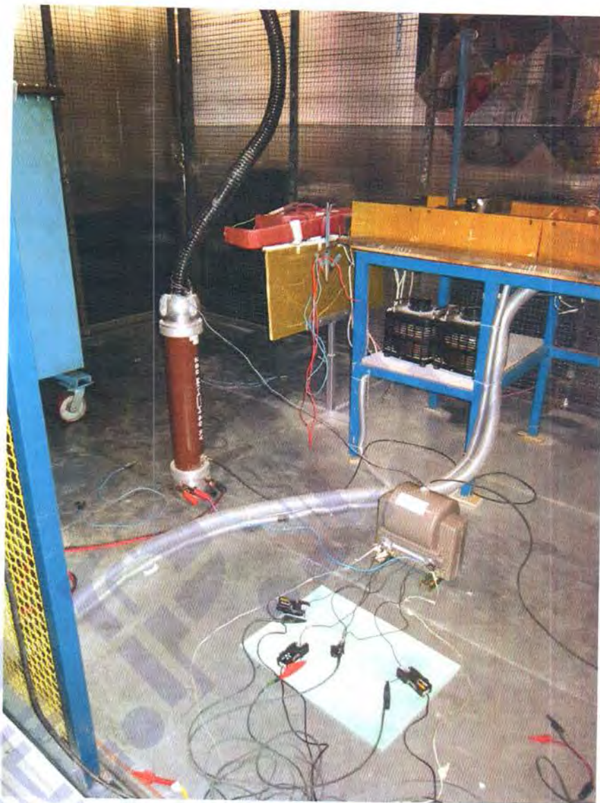
Figure 1: Installation of temperature rise test
